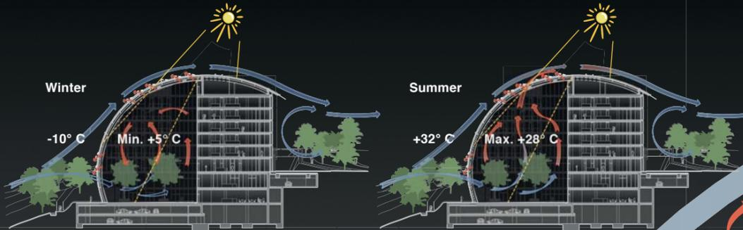
Building shape enhances venturi effect and supporting hot air exhaust on top of the grid shell
